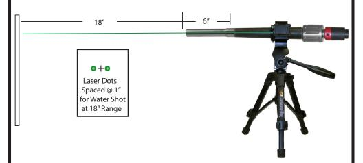
The Water Shot Barrel Extension adds 6" to the overall barrel length and extends the laser distance to 24" from the muzzle. The laser dots will be 1" apart at that distance but the center of the dots (as shown above) will always indicate the shot placement, at any distance.
