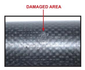
To repair a surface chip on the CarbonFire10 barrel, use a small amount of JB Weld epoxy putty to fill it in. Smooth out the area and let harden. Then sand lightly with a very fine grain sand paper to finish it. Do not sand into the carbon fiber.
