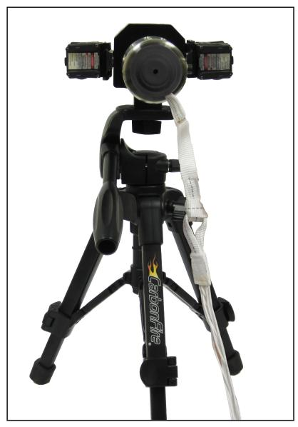
POSITION THE BARREL, AS SHOWN, WITHIN THE MOUNT TO INSURE THAT THE PARACHUTE CORD CLEARS THE TRIPOD AND MOUNT DURING EJECTION.
